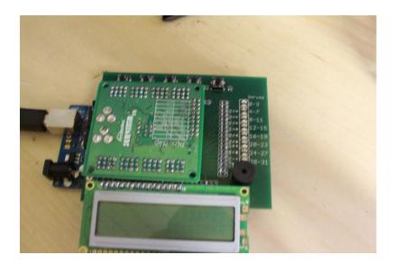
When plugged in to an active board, the EUT should have the green power LED on and pulse the red LED for 4-8 seconds, then shine bright red for 0.5 seconds, then off. The green LED will remain on.
